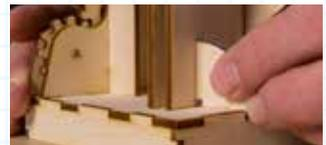
In engineering the word "square" means "at ninety degrees." Check square, using the included tool, any time you are assembling perpendicular surfaces like these.
