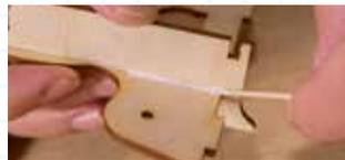
Lay glue into corners like these using the edge of your round toothpick. In this way, you can test-fit first and add glue second.
